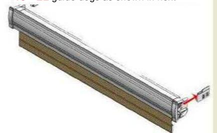
Locate guide dog flush to the head of the wall and the recess at the desired location. Push into position then hammer the masonry pins into position on each side
