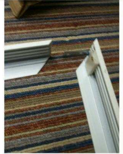
Insert corner brackets as shown in preparation to join the left and right element to the top element
