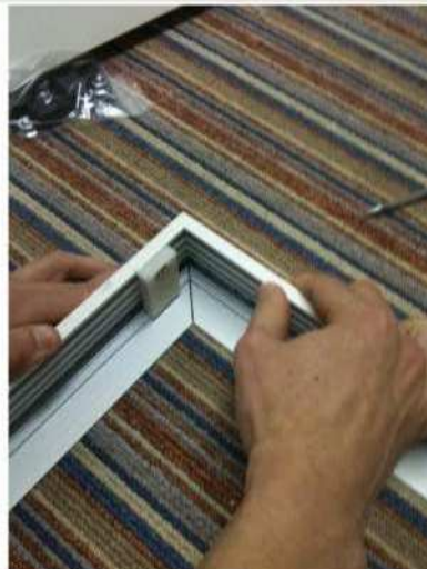
Join top element to left element via the corner bracket as shown by sliding the bracket into top slot
