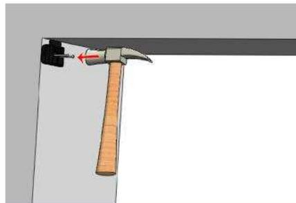
③ Mount cassette onto guide dogs and check level. This is done by lowering the blind to see if running off the square. If so, adjust using id guide dogs as shown in next step
