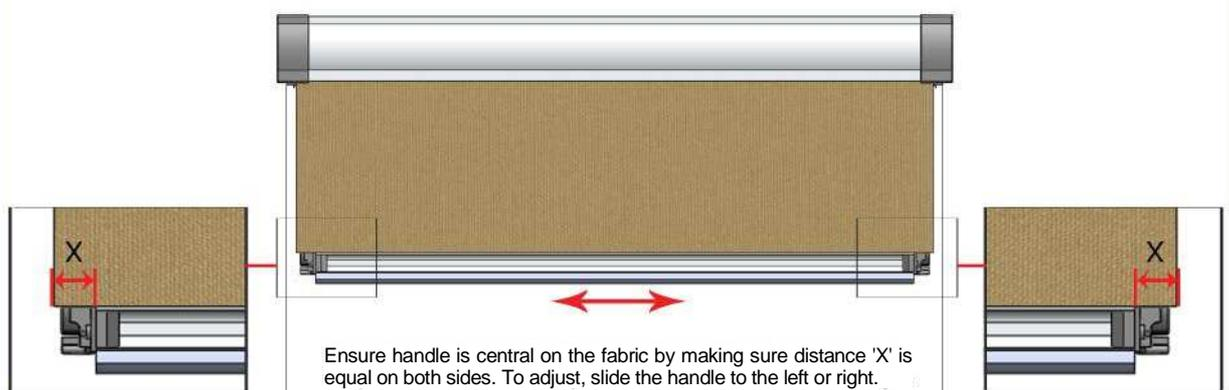
Ensure handle is central on the fabric by making sure distance 'X' is equal on both sides. To adjust, slide the handle to the left or right.
