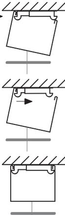
The brackets should compress and then allow the back of the blind to hook into the position shown
